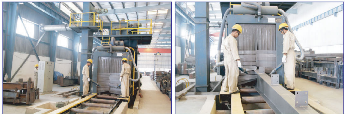
Shot Blasting of Built up Products
